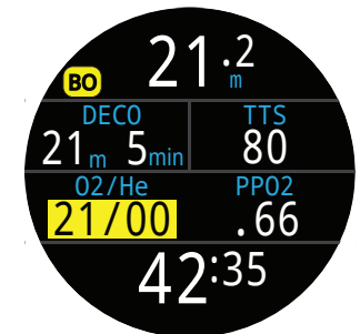
14. Gas Switch Required
